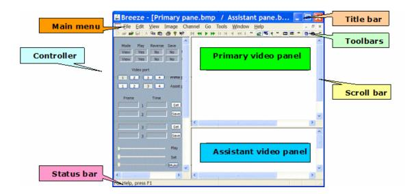
Primary and assistant video panels display video data. By default primary channel is connected via the video output port 1 to the primary video panel, and assistant channel is connected via the video output port 3 to the assistant video panel. But if it is necessary each video panel can be connected to any of 4 available video ports.
