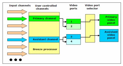
By default primary channel is connected via the video output port 1 to the primary video panel, and assistant channel is connected via the video output port 3 to the assistant video panel. But if it is necessary each video panel can be connected to any of 4 available video ports.
