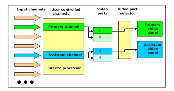
By default primary channel is connected via the video output port 1 to the primary video panel, and assistant channel is connected via the video output port 3 to the assistant video panel. But if it is necessary each video panel can be connected to any of 4 available video ports.
